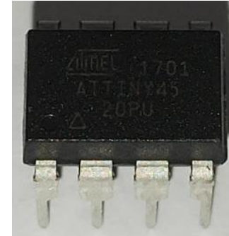
Watchdog Chip Attiny45-PU
